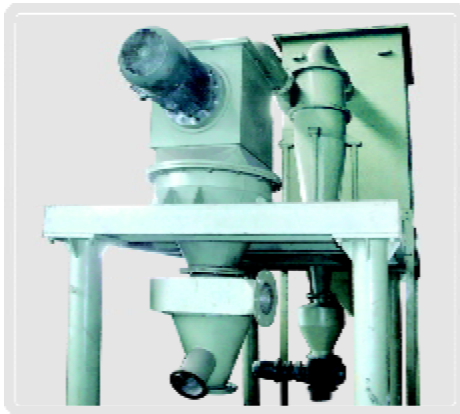
1 电 motor 2 classifying wheel 3 fine powder discharge 4 腔体 chamber 5 secondary air input 6 coarse material outlet
